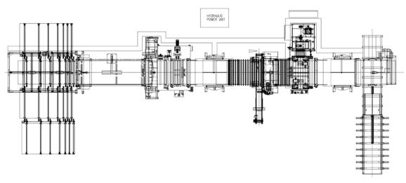
Electrolux Home Products recently purchased a CWP 60" x .060" x 25,000lb. Cut -to - Length system featuring a coil upender, coil storage rack, coil loading car, stock reel, B&K leveler, edge trimmer, threading tables, heavy duty 4 roll servo feed, mechanical shear, inspection conveyor, direct drop parts stacker and discharge conveyors for their new facility in Memphis, TN where they will be manufacturing cooking appliances.
