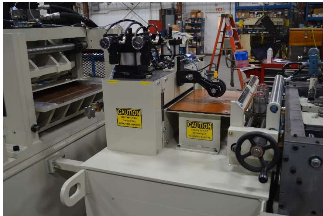
Servo feed with twist compensator and measuring wheel
