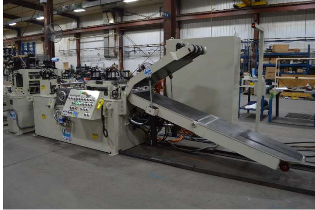
Coil processor with hold-down peeler station
