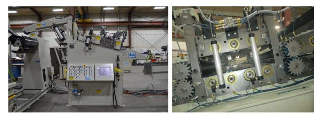
The ServoMax feed has powered passline height adjustment, a powered telescoping stock support table, and powered edge guides, all with push-button adjustment and automatic setup by job number. The feed is also equipped with automatic central lubrication for easy maintenance and anti-backup rolls for added safety. We also mounted the customer's Unist stock lubricator to the feed cabinet.
