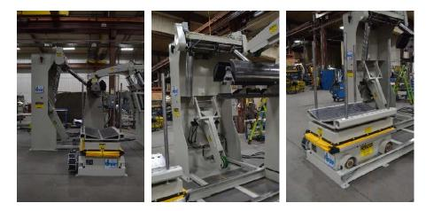
The powered straightener is equipped with our hold-down peeler station on the entry side for handsfree thread-up of coils and includes powered edge guides with push-button adjustment and automatic setup by job number. The straightener is equipped with automatic central lubrication for ease in maintenance and includes smooth chrome plated straightener rolls and our powered high lift head feature for ease in cleaning the straightener rolls between jobs.
