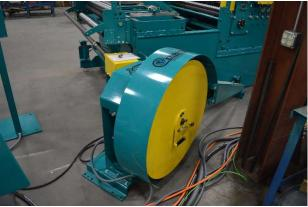
The beading roll embosses ridges into the sheet after straightening for rigidity of the finished product. A Dual Head Notcher includes 2 manually-adjusted "C" frame heads, each with a turret die to add a notch to each edge of the material. The notch is used to remove enough material to allow folding or forming of the part without the material buckling.
