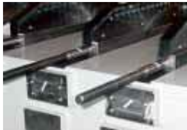
Lower wedge adjustment
