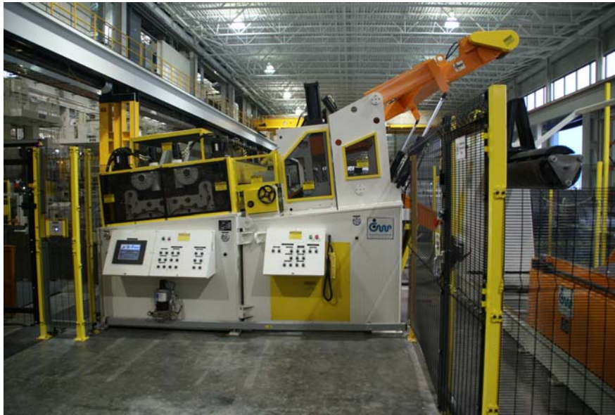
Model HD72-64/7PDS Heavy Duty Precision Power Driven Stock Straightener
