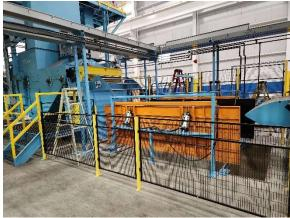
Our exclusive (4) roll servo feed guides the strip into our DieMation coil processor system, which includes (2) tooling stations servo controlled in both the X and Y axes and space to add more tooling stations in the future, and a scrap conveyor with scrap bin for the slugs. A second (4) roll feed is used to pull the strip through, and a hydraulic powered cutoff shear for blanking.
