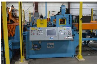
Parts exit the cutoff shear and drop onto a belt conveyor with a reject station that can drop parts into a scrap bin mounted under the conveyor. The direct drop stacker uses non-marking polyurethane fingers to support the parts and an air blower system for stacking light gauge materials, a scissor lift table with auto-down feature to minimize the drop distance, and end discharge conveyor with powered rollers to allow removal of stacks from either the end or the side of the conveyor
