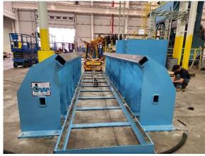
The (11) roll heavy-duty D series straightener includes chrome plated rolls, back-up flights on all work rolls, high rise upper rolls for access for cleaning, power to all straightener rolls, our powered handsfree cleaning system, and a hold-down peeler station for hands-free thread-up of coils. A set of powered pinch rolls pulls the strip through the customer's blast machine.
