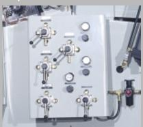
Popular and economical hand valve controls provide machine assist in the threading-up process of heavy and wide coil applications. Consolidated pushbutton and touch screen controls are optional.
