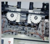
Heavy duty, power-driven split gear train distributes power evenly and efficiently to lower straightening rolls and entry/ exit pinch rolls.
