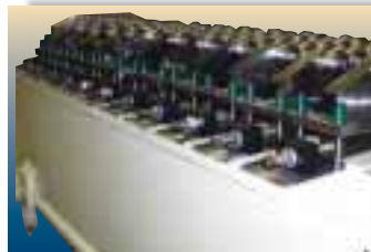
Fixed upper back-ups for greater leveling control
