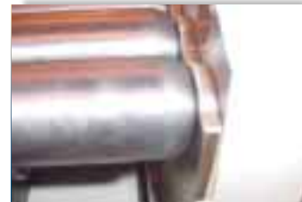
Floating full-width intermediate rolls
