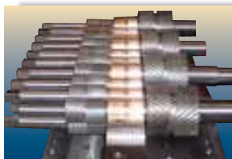
Dual herringbone gear train
